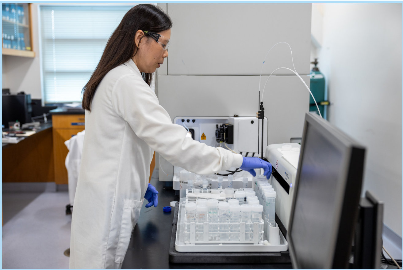
A DSRSD employee sets up an autosampler to test drinking water for lead and copper concentrations.
