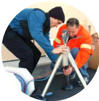
*The stainless steel impeller is fastened on to a 4-foot-tall tripod with rubber feet resting on the bottom of the tank reservoir.*
